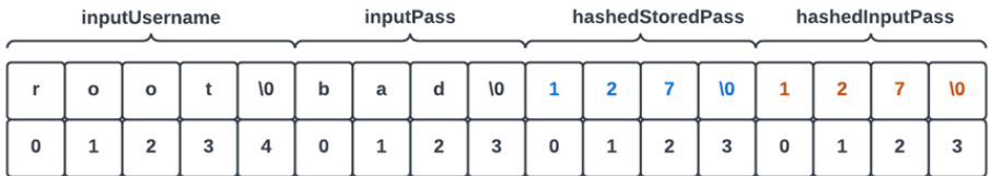
Figure 6: Memory layout after hashing the input password
